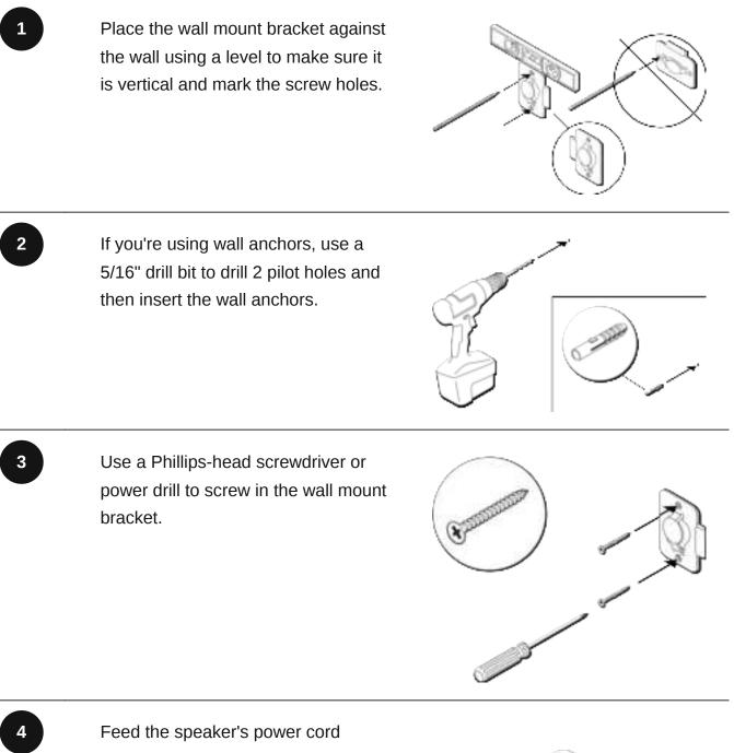
through the Mount opening and plug it into the speaker. Place it down onto the Mount.
