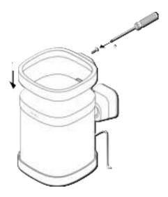
Slide the Mount down onto the wall bracket.
