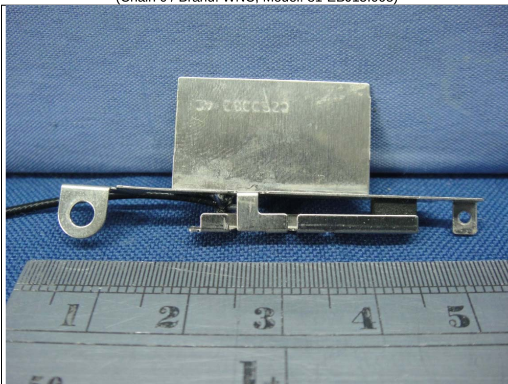
Antenna (Chain 0 / Brand: WNC, Model: 81-EBJ15.005)
