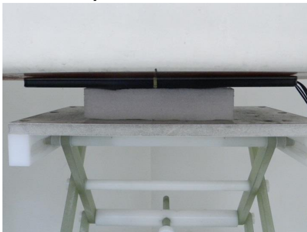
Bottom Face, Test Separation 0 mm
