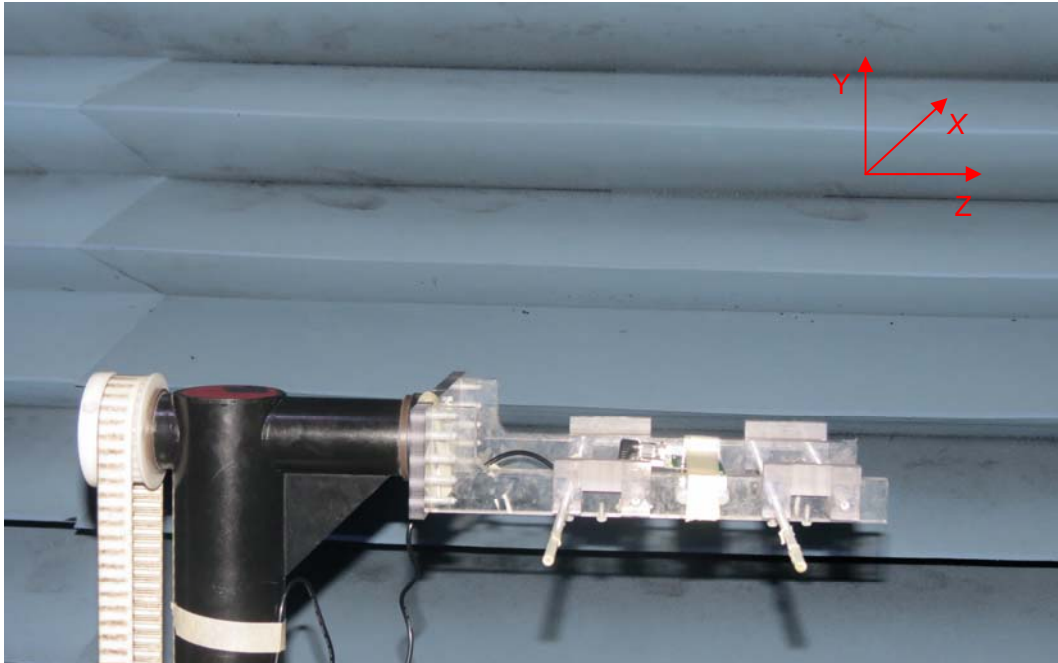
Picture 2: Typical Free Space EUT Mounting
