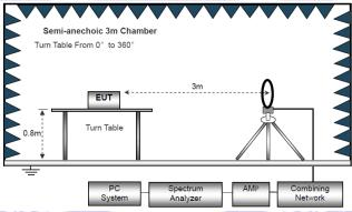
(B) Radiated Emission Test-Up Frequency 30MHz~1GHz
