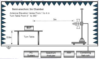
(C) Radiated Emission Test-Up Frequency Above 1GHz
