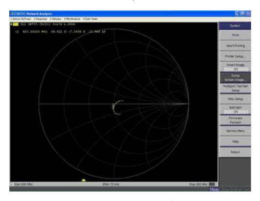
Measured impedance:  $48.611\Omega$ - $7.3j\Omega$
