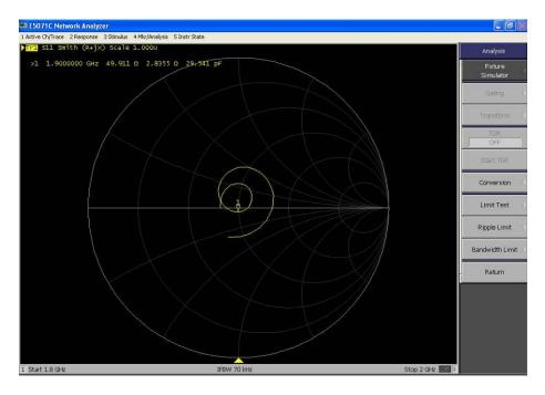
Measured impedance:  $49.911\Omega + 2.8j\Omega$
