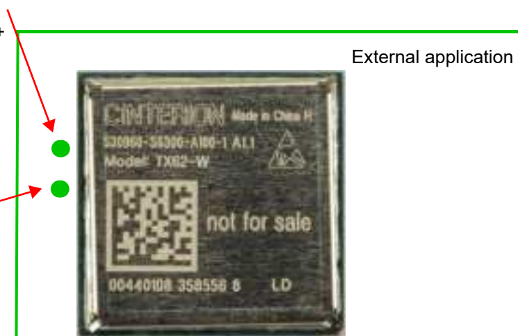
Figure 49: Position of reference points BATT+ and GND
