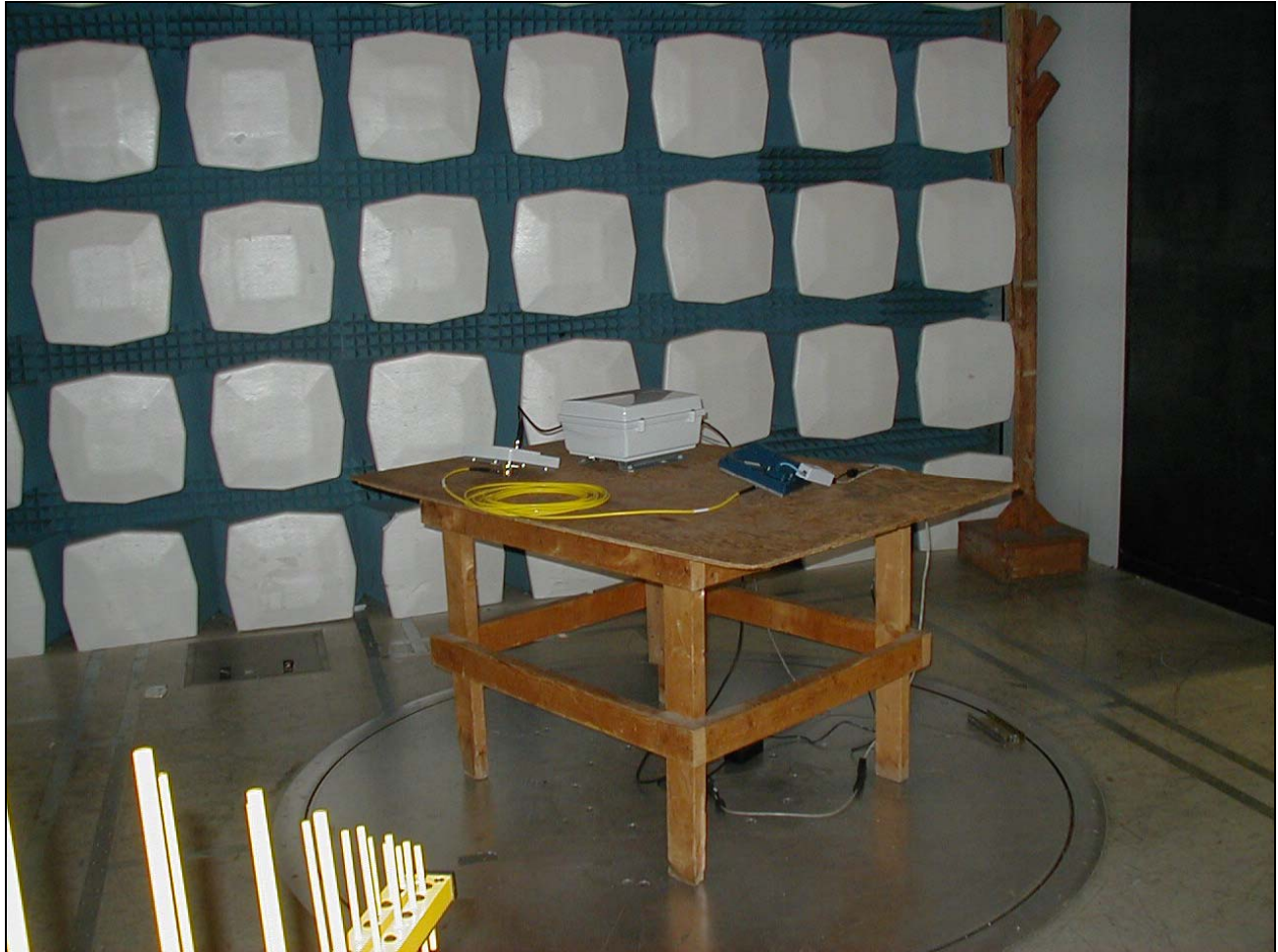
Photograph 2. Radiated Spurious Emissions, Test Set-up
