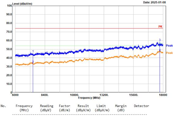
Condition: PK trace RBW:1MHz; VBW:3MHz; SWT:0.3sec AV trace RBW:1MHz; VBW:5kHz; SWT:auto
