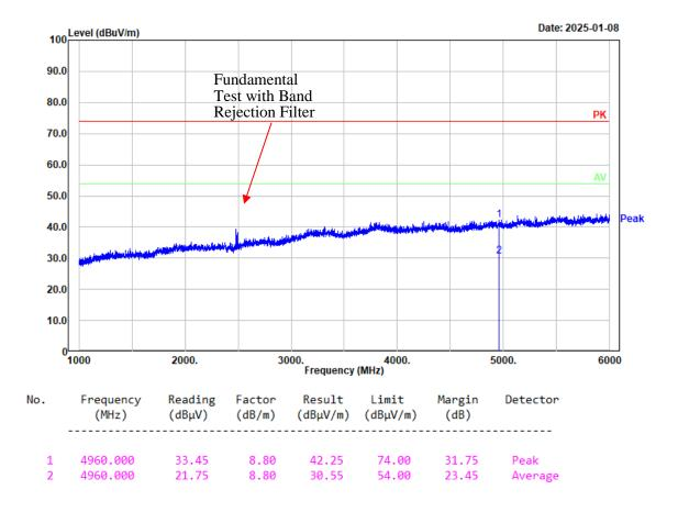
Project No.: 2403A43118E-RF Tester: Tao Zhu Condition: PK trace RBW:1MHz; VBW:3MHz; SWT:0.3sec Polarization: vertical Note: BLE 1M High Channel 2480MHz Chain 0
