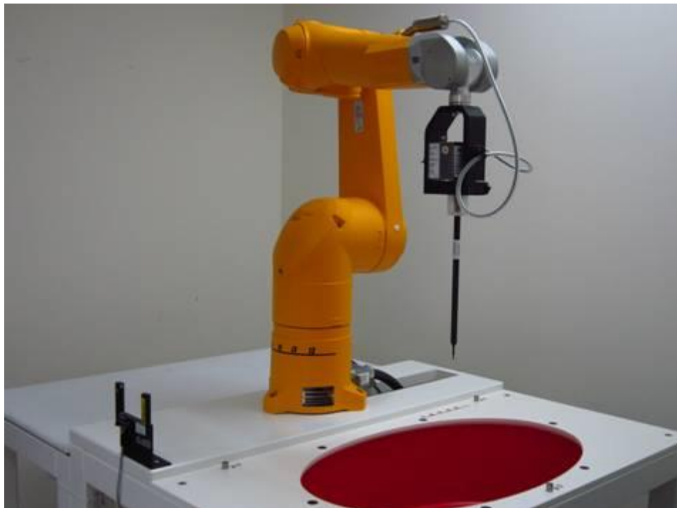
Fig.1 Photograph of the SAR measurement system
