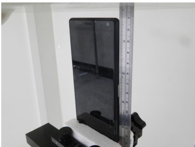
Top Side, Test Separation 10 mm
