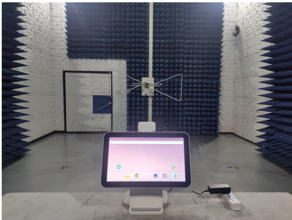
FCC RADIATED EMISSION TEST SETUP ABOVE 1GHZ
