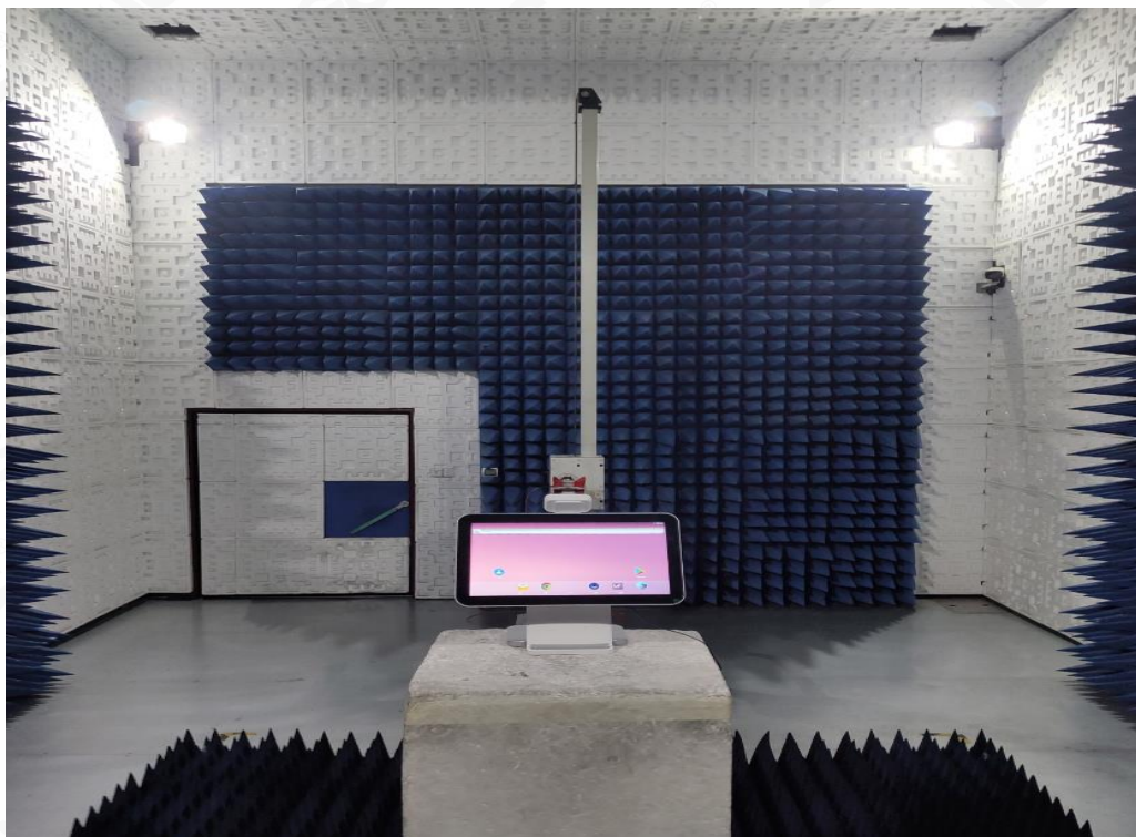
FCC RADIATED EMISSION TEST SETUP ABOVE 1GHZ
