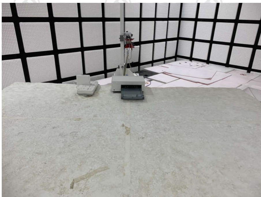
Radiated spurious emission Test Setup-2(Above 1GHz)
