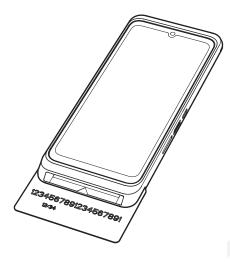
The device supports both magnetic stripe cards and smart cards. To carry out how to use a magnetic stripe card follow these steps:
