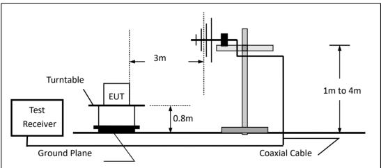
(c) For radiated emissions above 1000MHz
