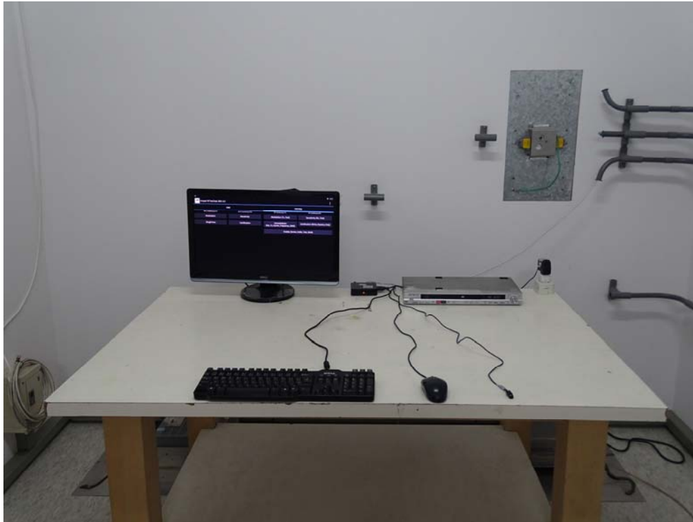
Front View of Conducted Test
