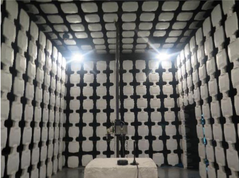
Pic3. Radiated spurious emissions (Above 1GHz)
