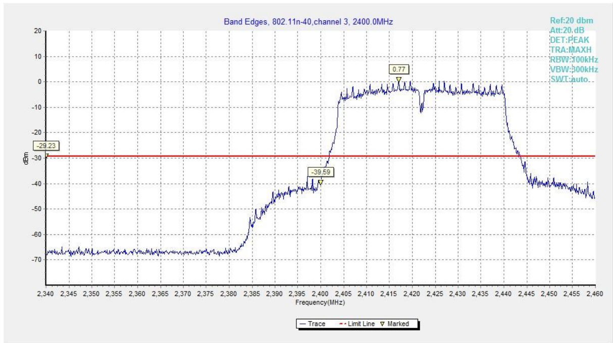
Fig.31 Band Edges (802.11n HT40, CH 3)
