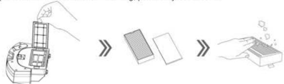
Wash the dust box and primary filter, air the dust box and filter assembly, and keep dry to ensure their service life.
