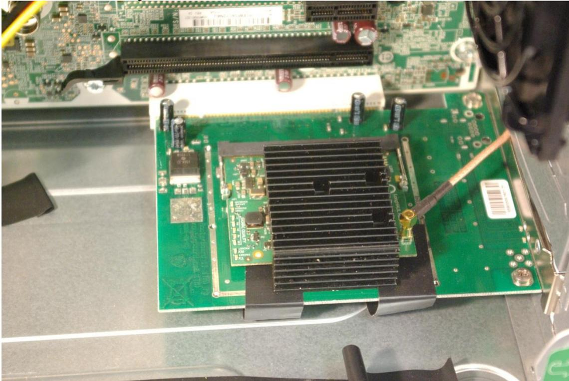
Transmitter in place on support PCI interface board
