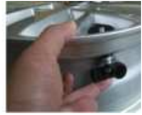
① Remove the tire ② Cut off the original valve of the car ③ Clean the valve hole ④ Installing sensors
