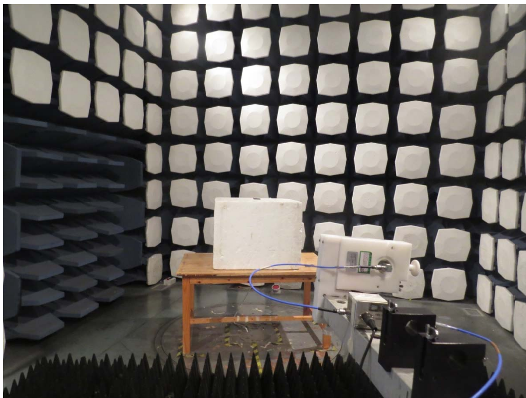
Picture 1: Radiated Spurious Emissions Test setup
