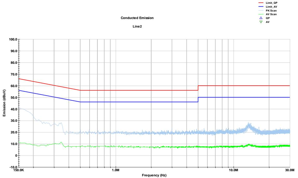
\*Test has been executed on AC/DC adapter of auxiliary equipment LENOVO T430 laptop PC.
