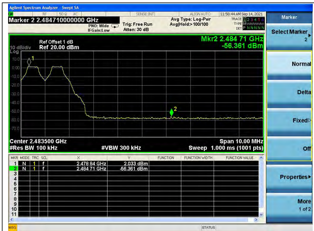
(Band edge with hopping on, Channel 78, GFSK)
