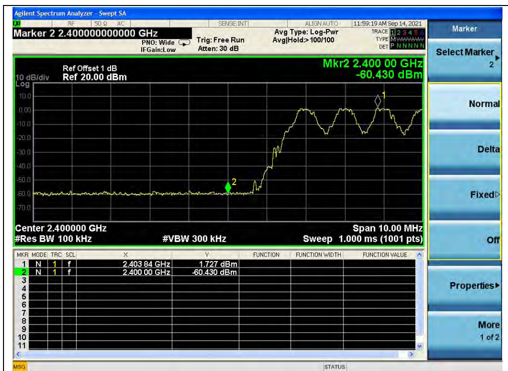
(Band edge with hopping on, Channel 0, GFSK)
