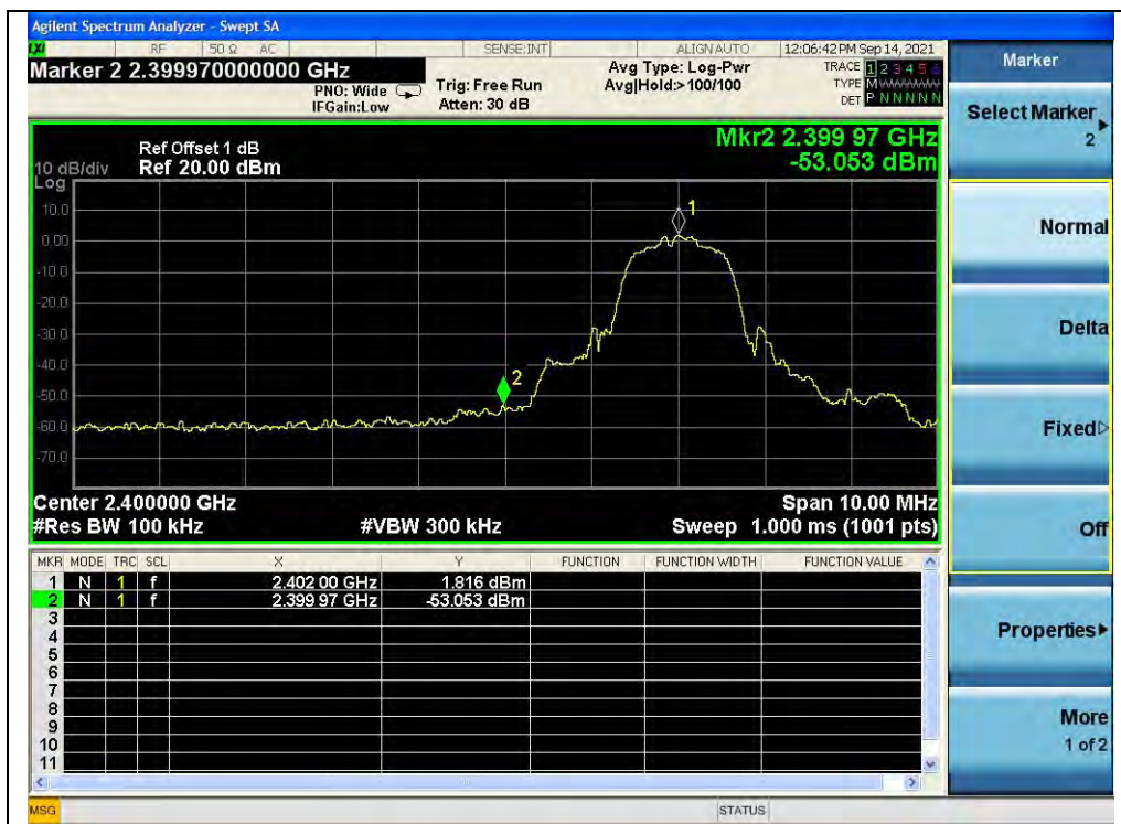
(Band edge, Channel 0, \pi/4 -DQPSK)
