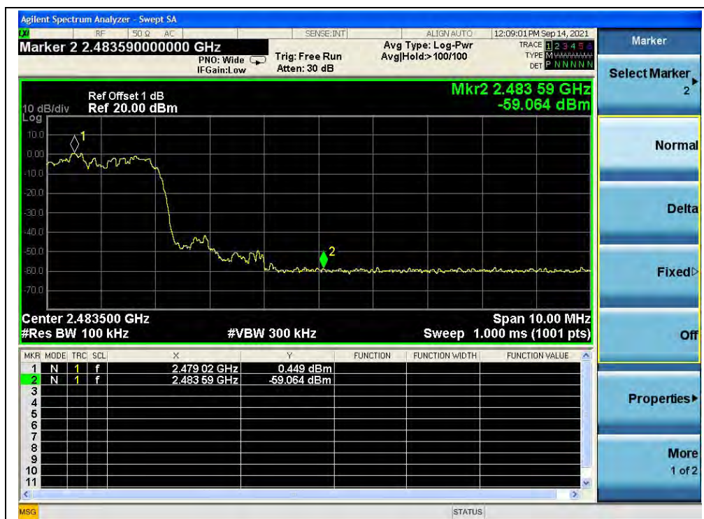
(Band edge with hopping on, Channel 78, 8-DPSK)
