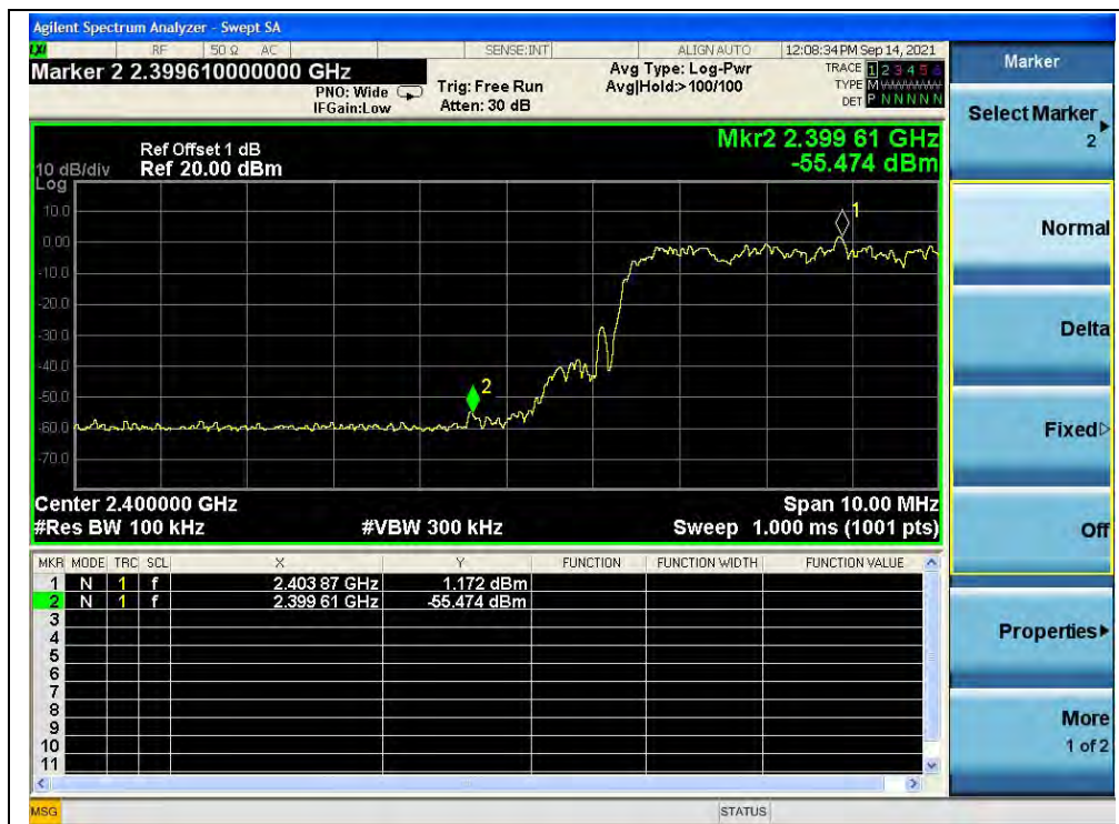
(Band edge with hopping on, Channel 0, 8-DPSK)
