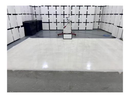
**Set-up for Radiated Spurious Emission, Above 1GHz**
