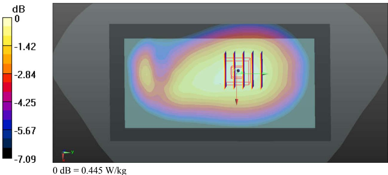
**30\_LTE Band 13\_10M\_QPSK\_1RB\_25Offset\_Back\_10mm\_Ch23230**
