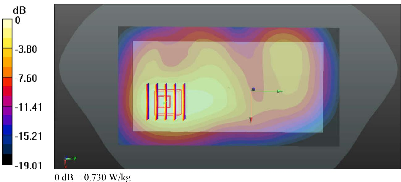
**29\_LTE Band 12\_10M\_QPSK\_1RB\_25Offset\_Back\_10mm\_Ch23095**
