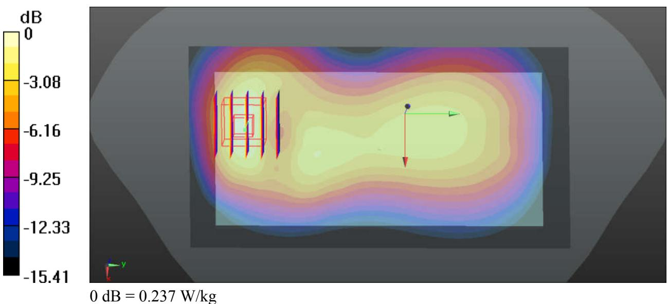
**31\_LTE Band 5\_10M\_QPSK\_1RB\_25Offset\_Back\_10mm\_Ch20525**
