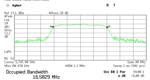
Transmit Freq Error -69.705 kHz x dB Bandwidth 15.890 MHz
