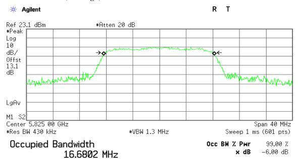
Transmit Freq Error -50.198 kHz x dB Bandwidth 16.193 MHz
