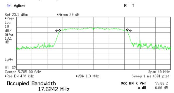
Transmit Freq Error -20.992 kHz x dB Bandwidth 17.275 MHz
