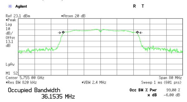
Transmit Freq Error -106.911 kHz x dB Bandwidth 35.762 MHz
