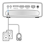
2 When connecting to the headphones, use the volume control on the remote control to adjust the volume to a comfortable level.
