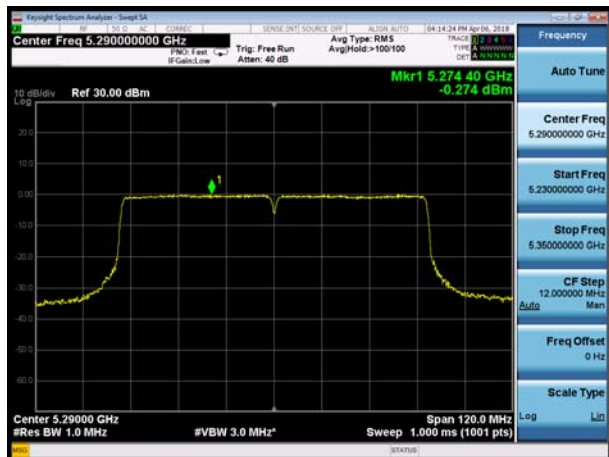
U-NII-2A, 802.11ac VHT80, Channel No.: 58
