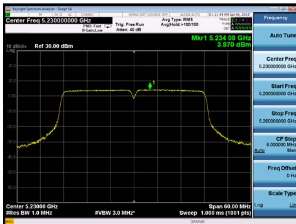
U-NII-1, 802.11ac VHT80, Channel No.: 42
