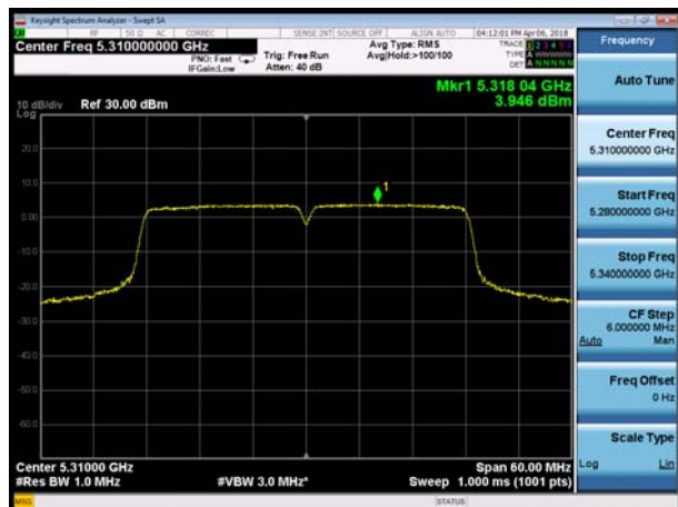
U-NII-2A, 802.11ac VHT80, Channel No.: 58
