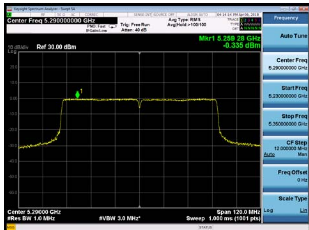
U-NII-2A, 802.11ac VHT80, Channel No.: 58
