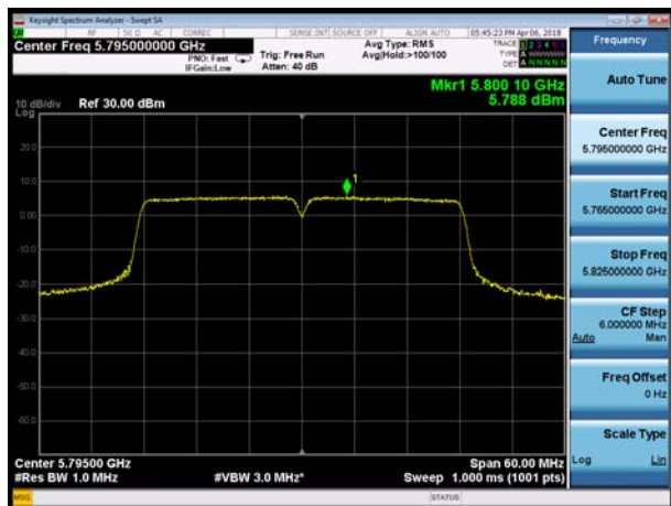
U-NII-3, 802.11ac VHT80, Channel No.: 155
