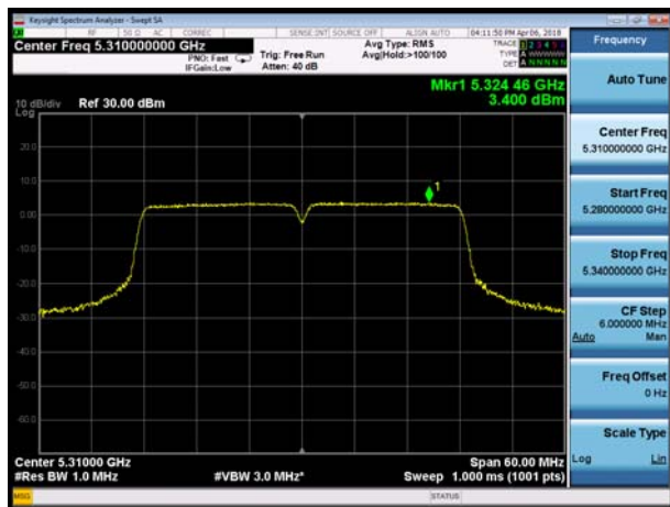
U-NII-2A, 802.11ac VHT80, Channel No.: 58
