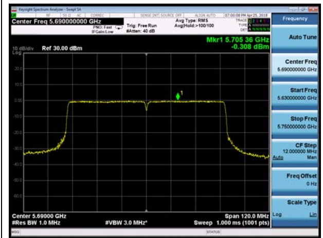
U-NII-2C, 802.11ac VHT80, Channel No.: 138
