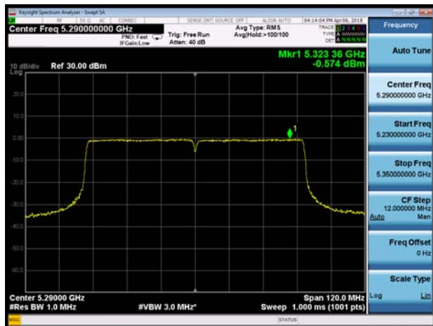
U-NII-2A, 802.11ac VHT80, Channel No.: 58
