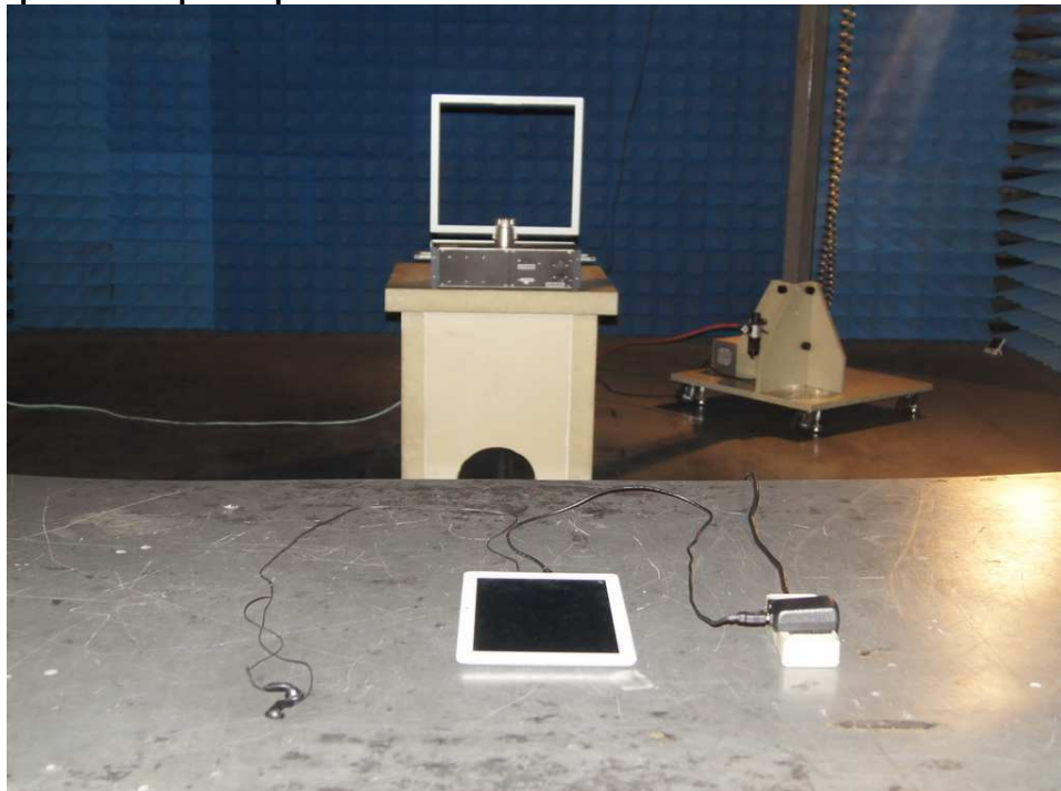
Photograph 2: Set-up for Spurious Emissions below 30MHz
