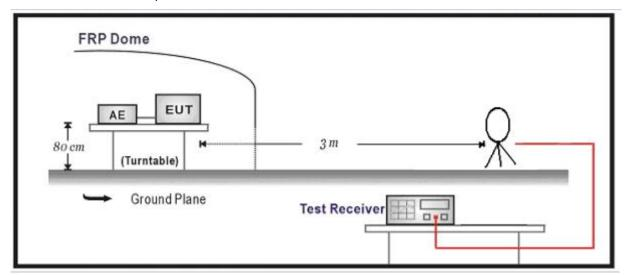
Below 1GHz Test Setup:
