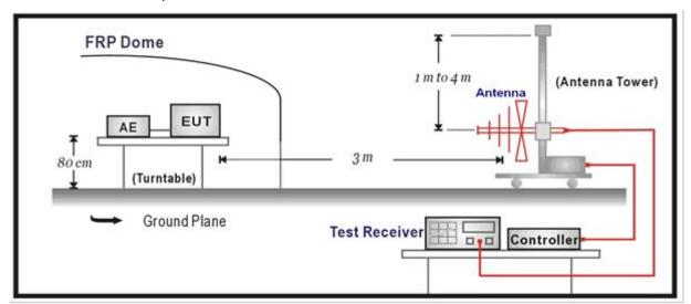
Above 1GHz Test Setup:
