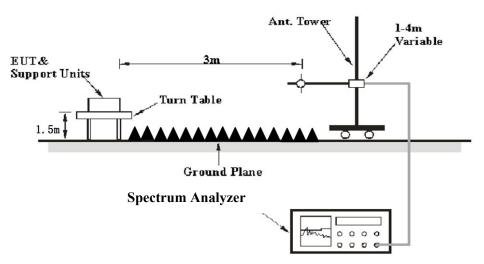
The radiated emission tests were performed in the 3meters test site, using the setup accordance with the ANSI C63.10-2013. The specification used was the FCC 15.205, FCC 15.209, FCC 15.247, RSS-Gen and RSS-247 limits.
