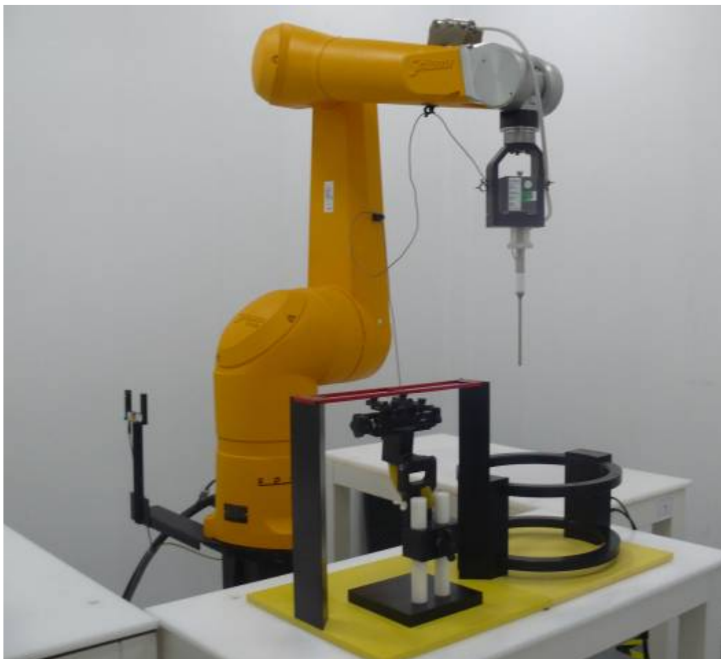
Picture 1: HAC T-Coil System Layout
