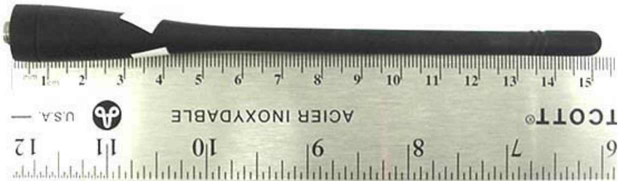
Whip Antenna (P/N: KRA-27M)
