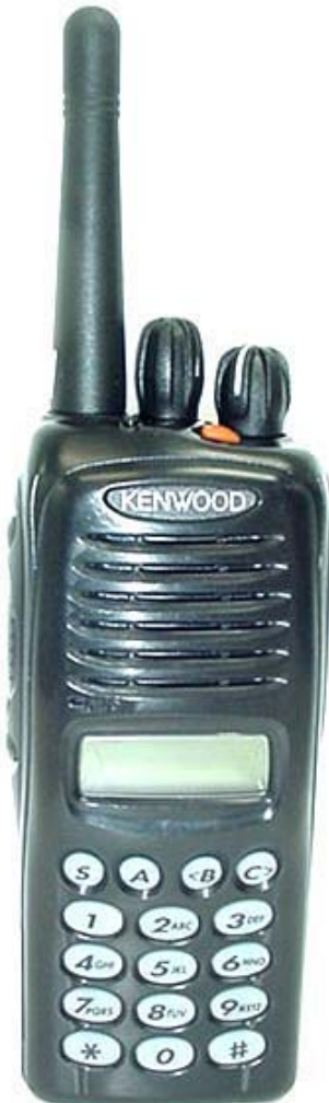
Front of DUT Stubby Antenna (P/N: KRA-23)
