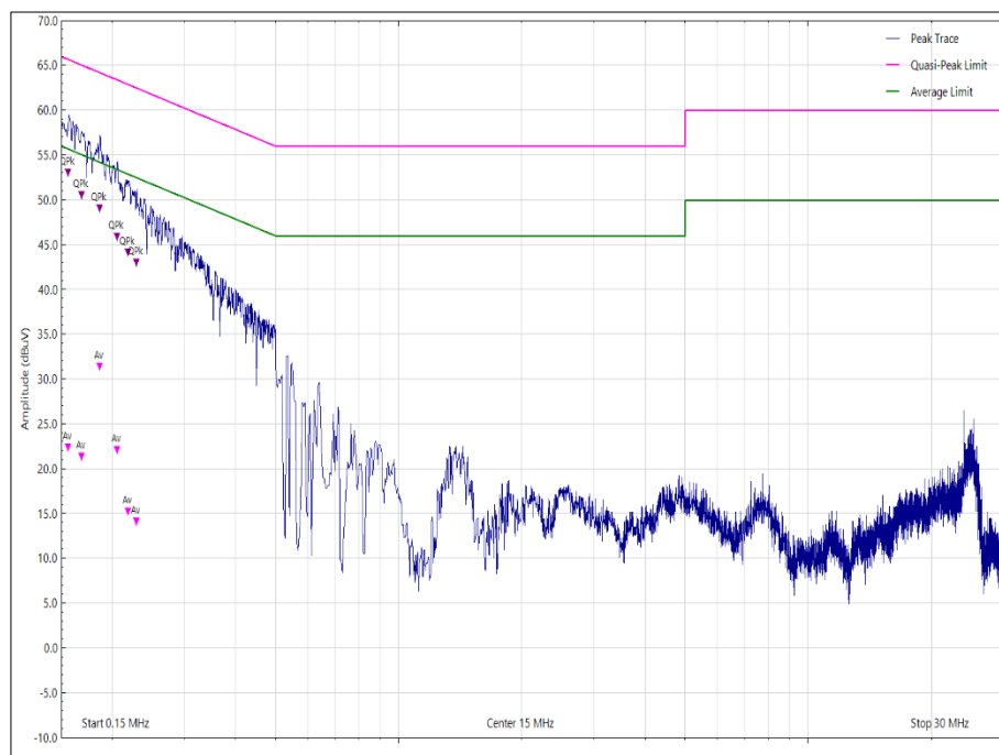
Figure 5 - Neutral Line - 150 kHz to 30 MHz
