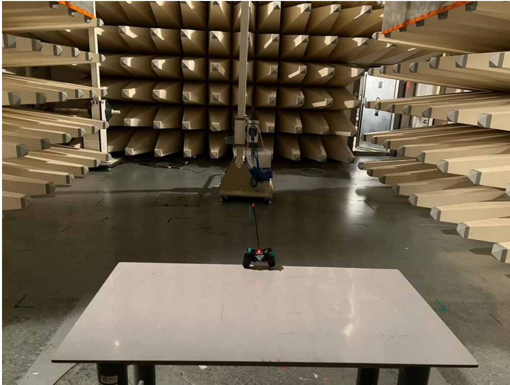
Set-up of Radiation Emission from 200 – 1000MHz
