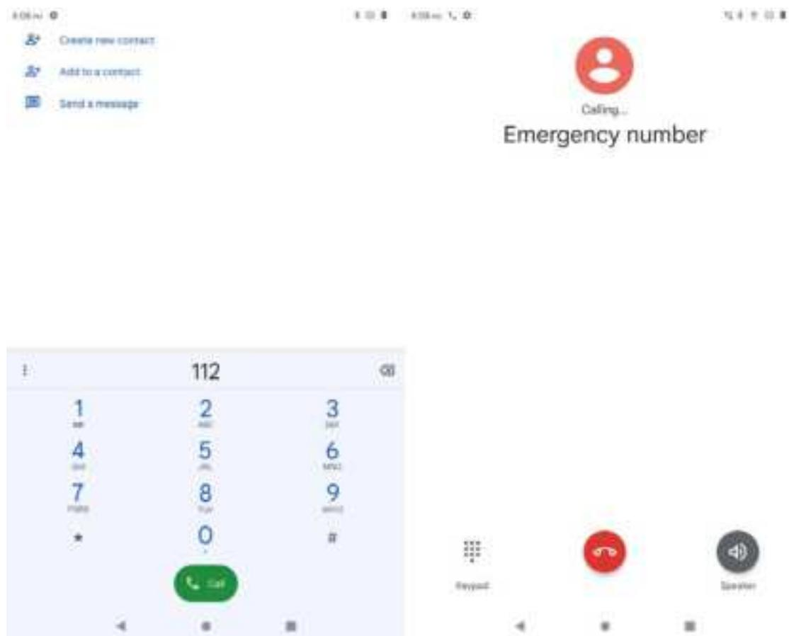
**Note:** *Emergency Call is possible without SIM card. The loudspeaker must be switched on or a headphone must be connected.*
