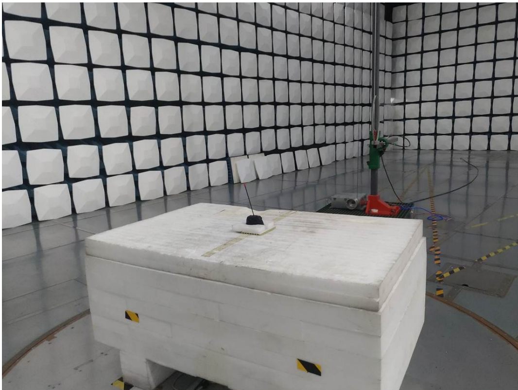
Radiated Emission 9k-30MHz Perpendicular View
