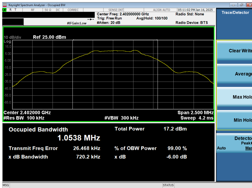
Plot 7-1. 6dB BW & 99% OBW Plot Antenna WF8 (Bluetooth (LE), 1Mbps, iPA – Ch. 0)
