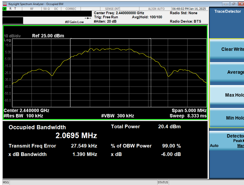
Plot 7-23. 6dB BW & 99% OBW Plot Antenna WF7b (Bluetooth (LE), 2Mbps, iPA – Ch. 19)
