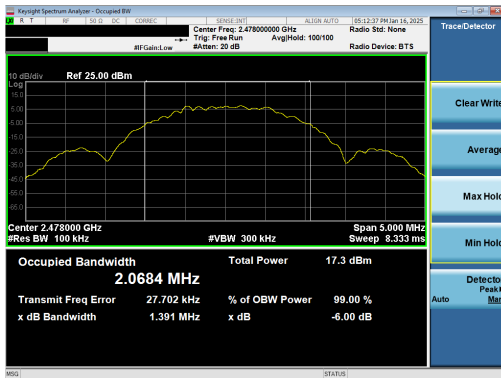
Plot 7-6. 6dB BW & 99% OBW Plot Antenna WF8 (Bluetooth (LE), 2Mbps, iPA – Ch. 38)
