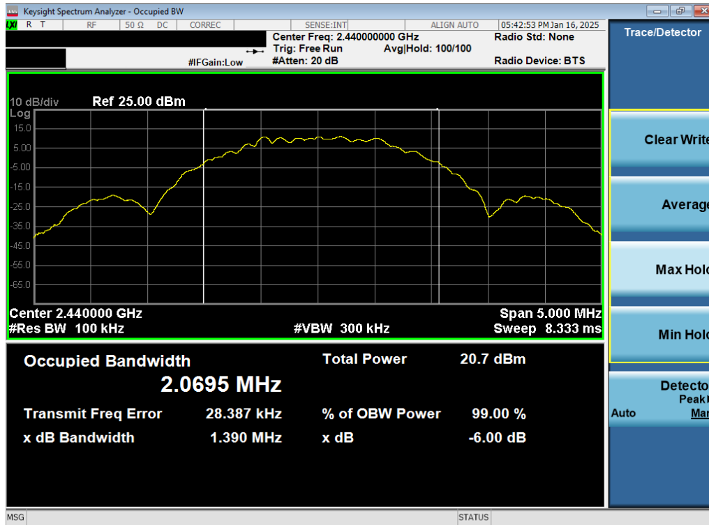
Plot 7-11. 6dB BW & 99% OBW Plot Antenna WF8 (Bluetooth (LE), 2Mbps, iPA – Ch. 19)
