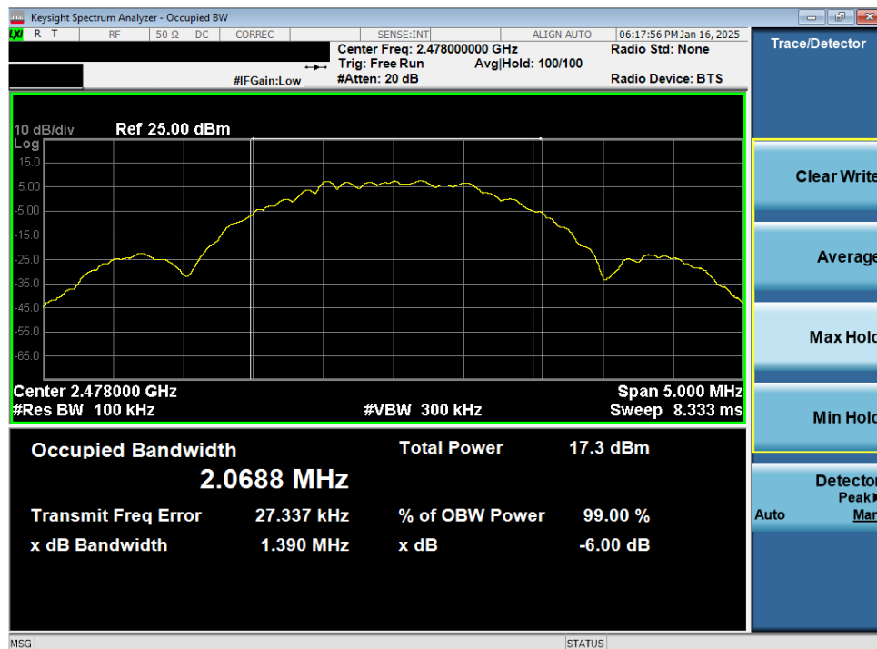
Plot 7-18. 6dB BW & 99% OBW Plot Antenna WF7b (Bluetooth (LE), 2Mbps, iPA – Ch. 38)
