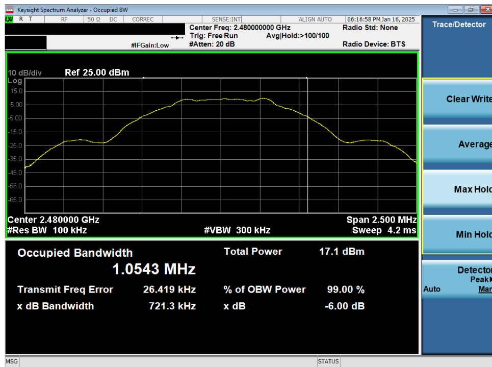
Plot 7-15. 6dB BW & 99% OBW Plot Antenna WF7b (Bluetooth (LE), 1Mbps, iPA – Ch. 39)
