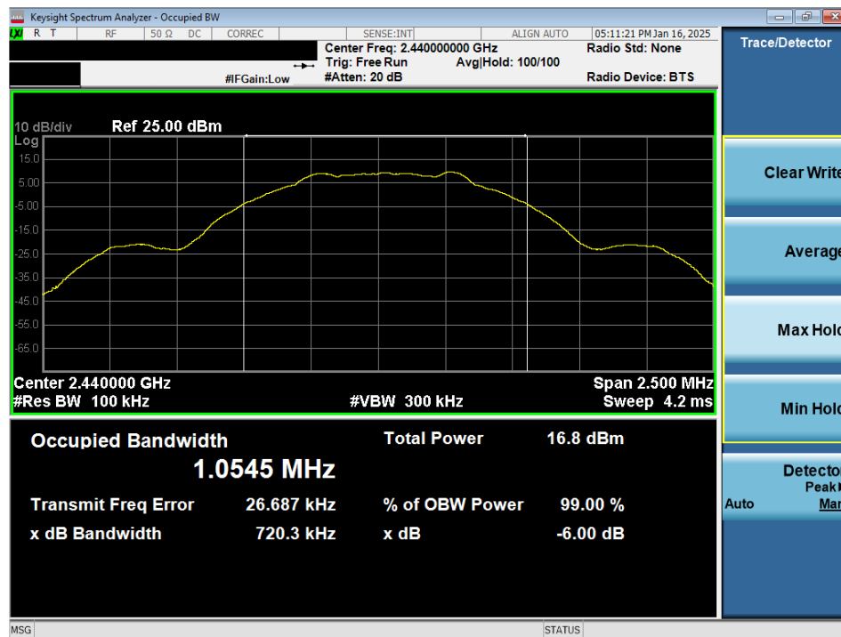
Plot 7-2. 6dB BW & 99% OBW Plot Antenna WF8 (Bluetooth (LE), 1Mbps, iPA – Ch. 19)
