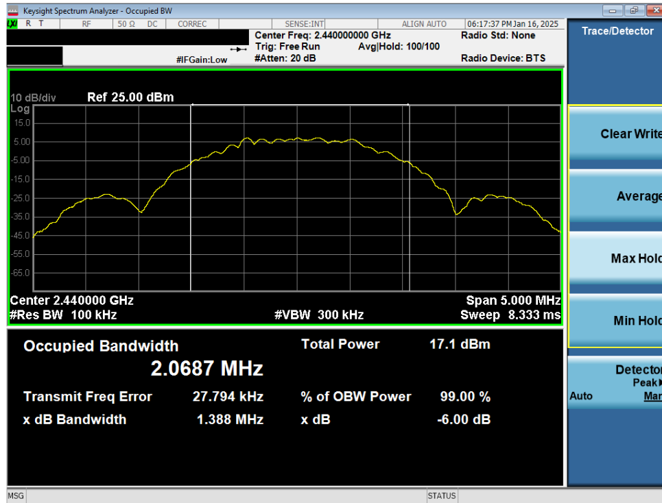
Plot 7-17. 6dB BW & 99% OBW Plot Antenna WF7b (Bluetooth (LE), 2Mbps, iPA – Ch. 19)
