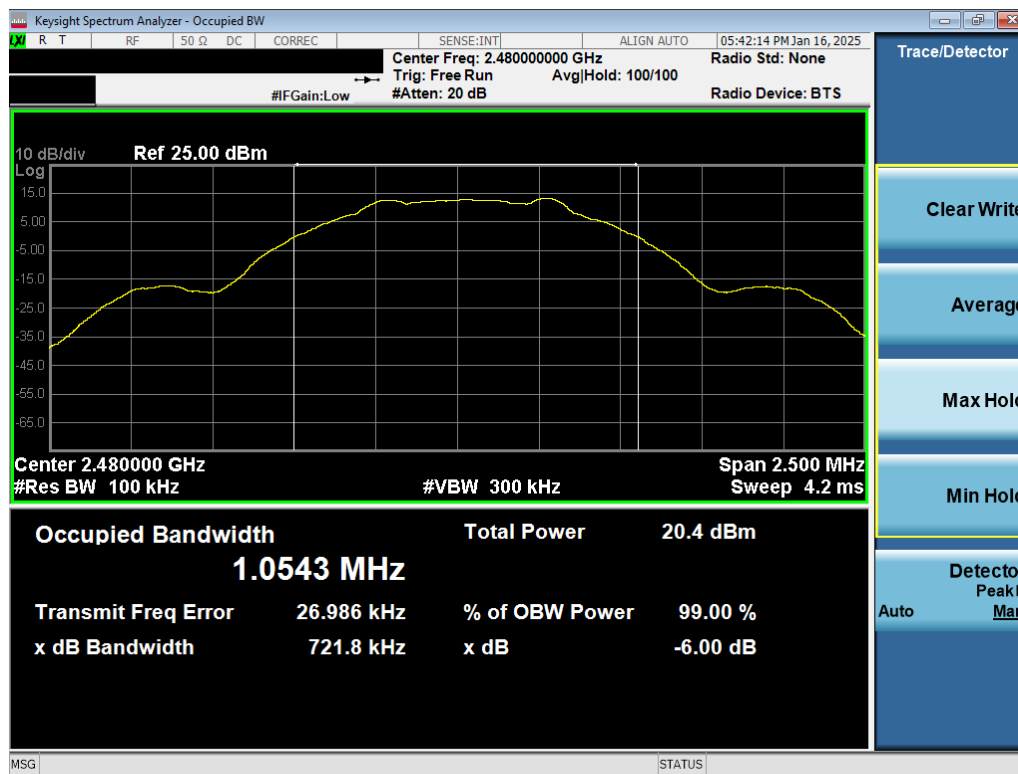
Plot 7-9. 6dB BW & 99% OBW Plot Antenna WF8 (Bluetooth (LE), 1Mbps, iPA – Ch. 39)
