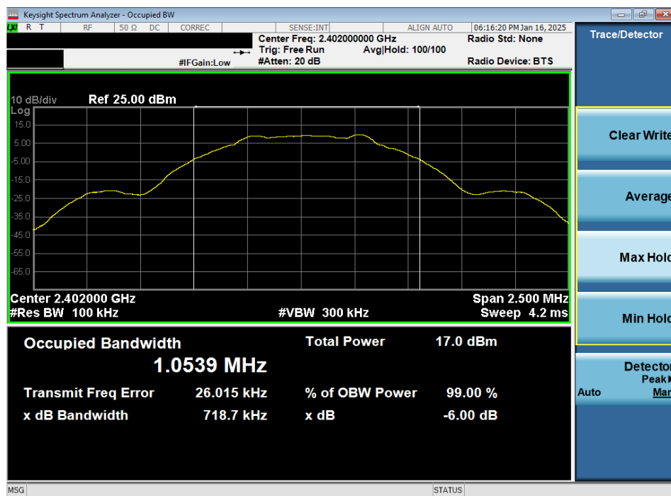
Plot 7-13. 6dB BW & 99% OBW Plot Antenna WF7b (Bluetooth (LE), 1Mbps, iPA – Ch. 0)
