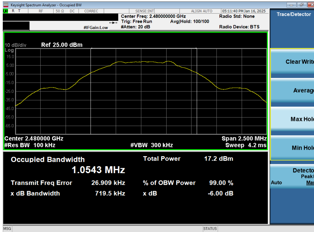
Plot 7-3. 6dB BW & 99% OBW Plot Antenna WF8 (Bluetooth (LE), 1Mbps, iPA – Ch. 39)
