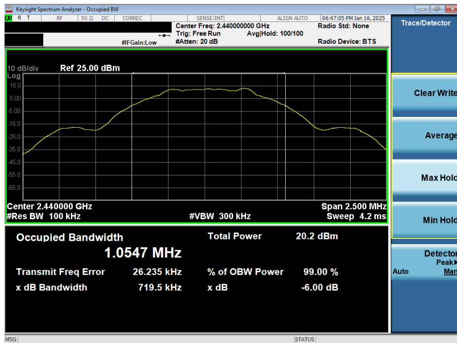
Plot 7-20. 6dB BW & 99% OBW Plot Antenna WF7b (Bluetooth (LE), 1Mbps, iPA – Ch. 19)
