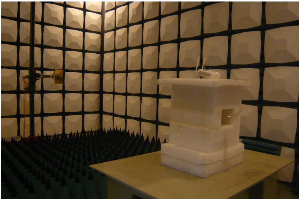
Radiated Emission Above 1GHz View
