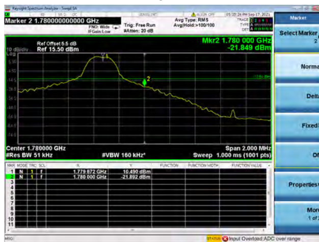
Band66 / 5MHz / High CH / QPSK / 1 RB
