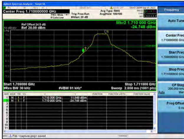
Band4 / 1.4MHz / High CH / QPSK / 1 RB
