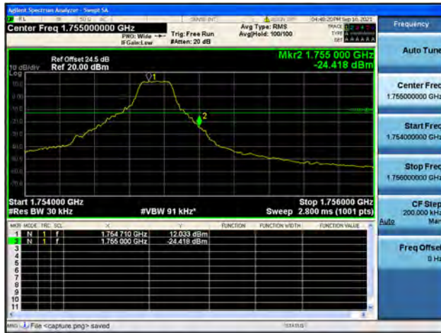
Band4 / 1.4MHz / High CH / QPSK / 1 RB
