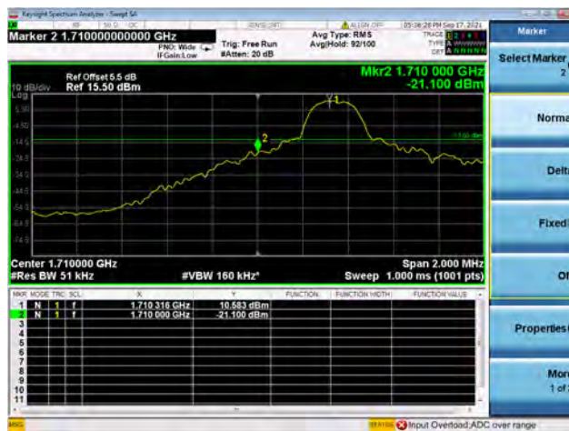
Band66 / 5MHz / High CH / QPSK / 1 RB
