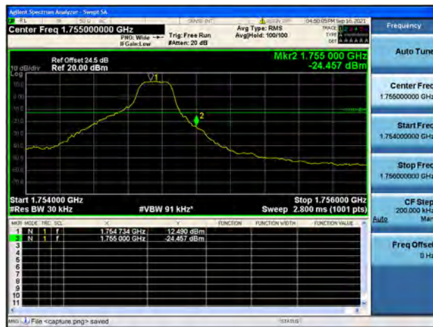
Band4 / 3MHz / High CH / QPSK / 1 RB
