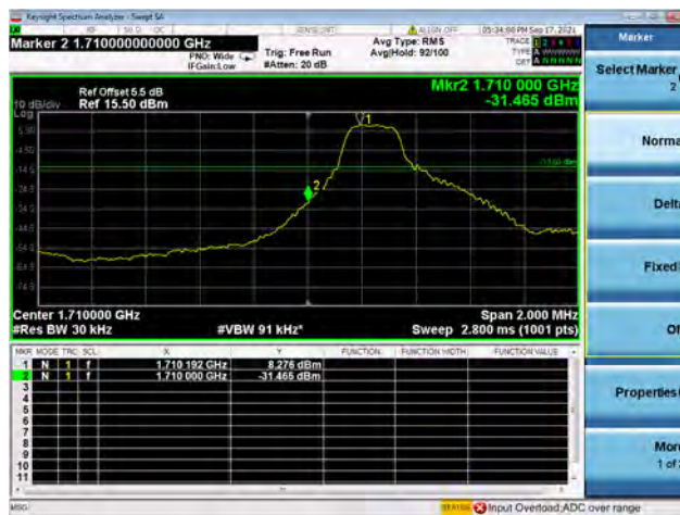
Band66 / 3MHz / High CH / QPSK / 1 RB
