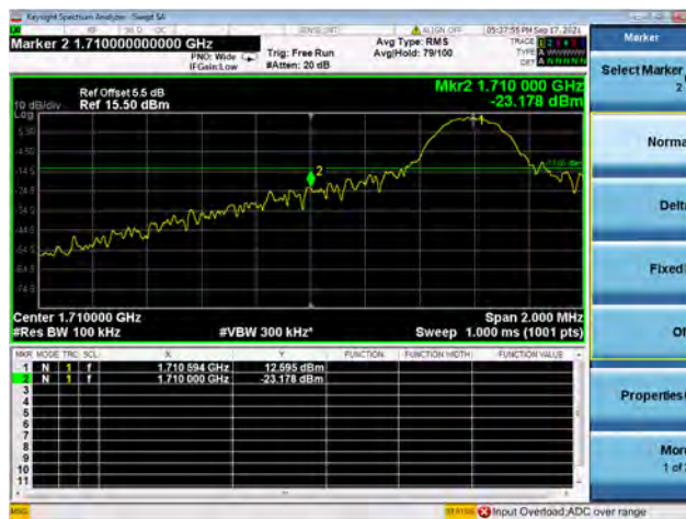
Band66 / 10MHz / High CH / QPSK / 1 RB
