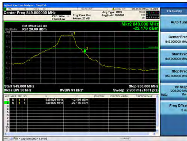
Band5 / 3MHz / High CH / QPSK / 1 RB
