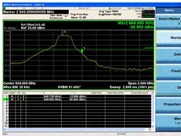
Band26 / 3MHz / High CH / QPSK / 1 RB
