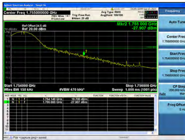
Band4 / 15MHz / High CH / QPSK / 1 RB
