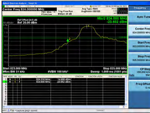
Band5 / 5MHz / High CH / QPSK / 1 RB
