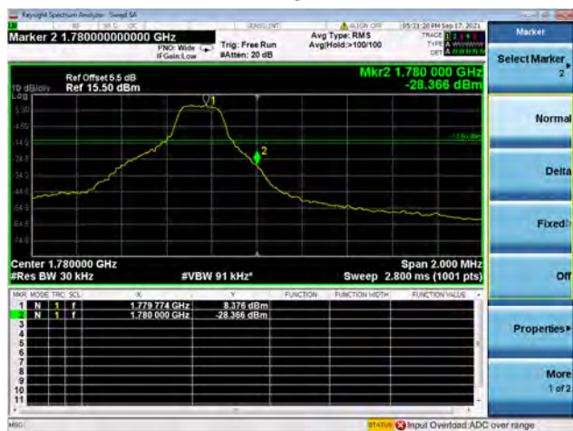
Band66 / 1.4MHz / High CH / QPSK / 1 RB
