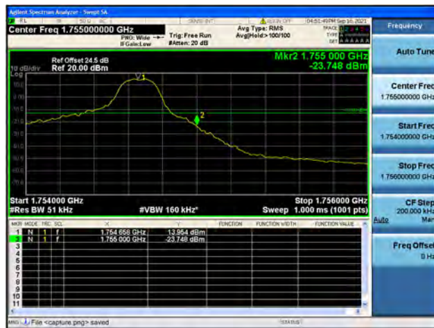
Band4 / 5MHz / High CH / QPSK / 1 RB
