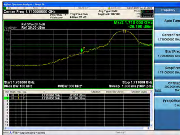
Band4 / 10MHz / High CH / QPSK / 1 RB
