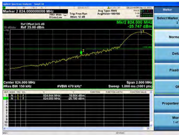
Band26 / 15MHz / High CH / QPSK / 1 RB
