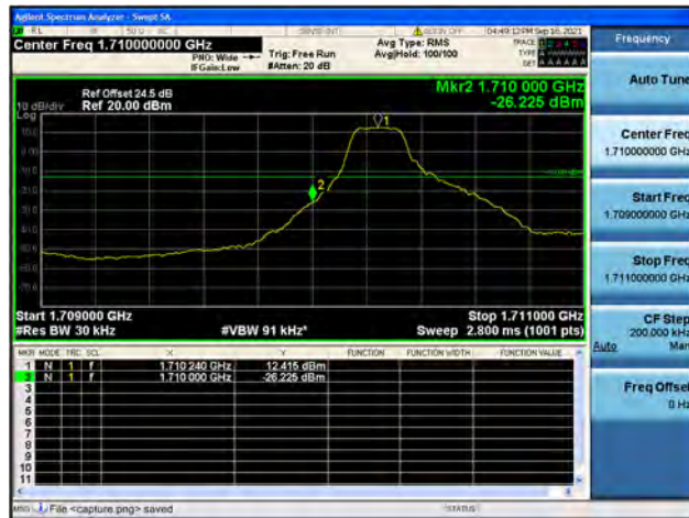
Band4 / 3MHz / High CH / QPSK / 1 RB
