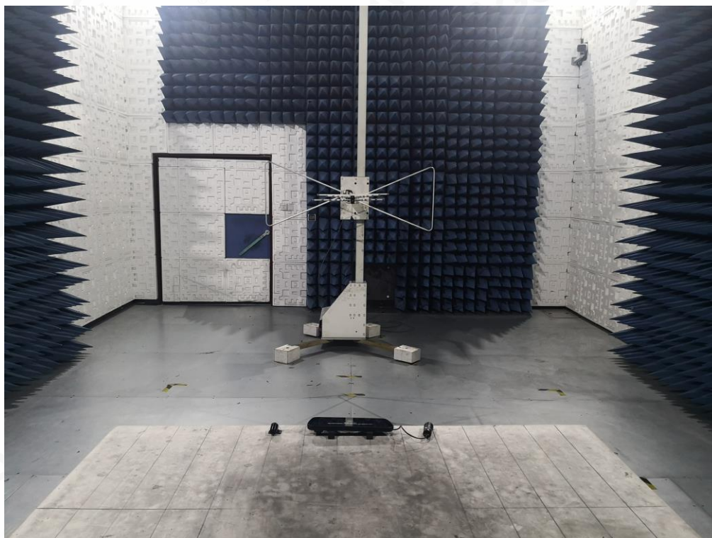
FCC RADIATED EMISSION TEST SETUP ABOVE 1GHZ
