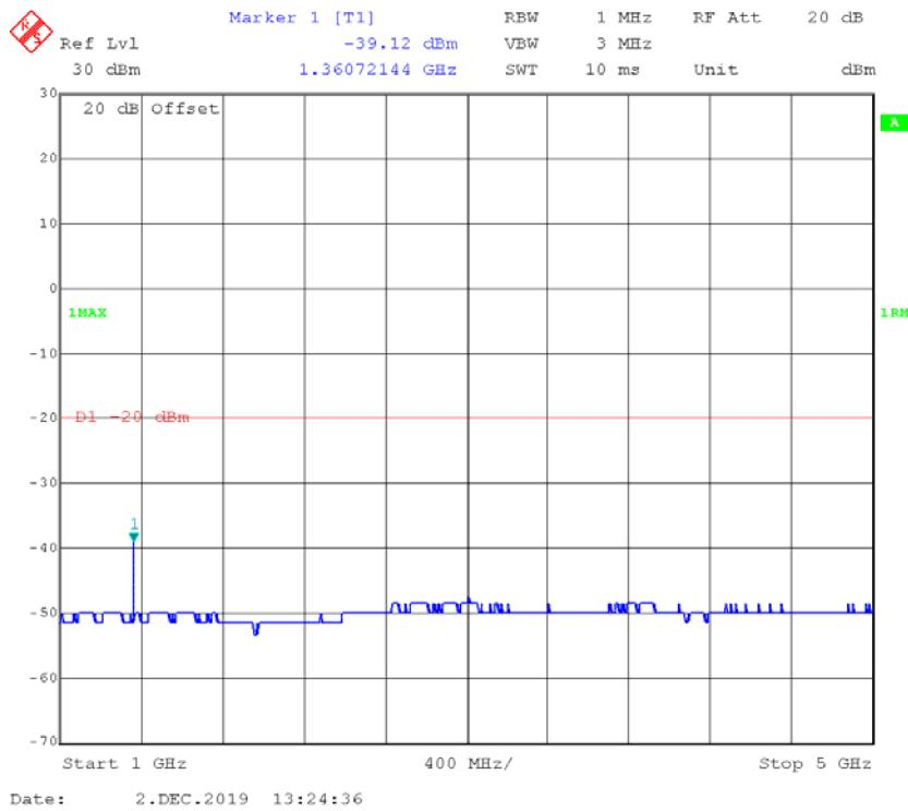
**12.5kHz,4FSK, High power, 455.0125 MHz**
