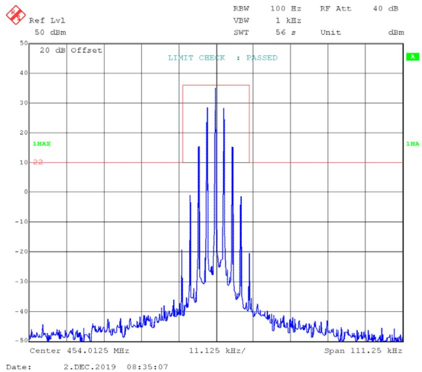
**FM,12.5kHz,Low Power - Frequency 454.0125 MHz:****99% Occupied & 26 dB Bandwidth**
