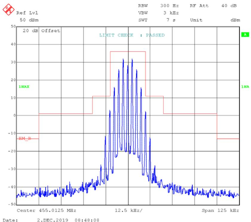
**FM,25kHz,Low Power - Frequency 455.0125 MHz:****99% Occupied & 26 dB Bandwidth**
