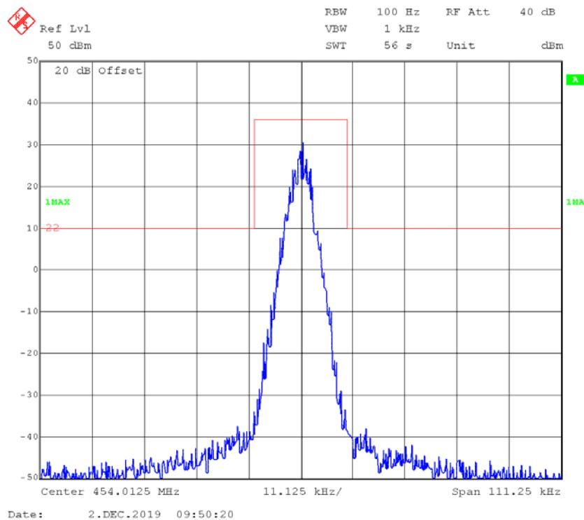
**4FSK,12.5kHz,Low Power - Frequency 454.0125 MHz:****99% Occupied & 26 dB Bandwidth**
