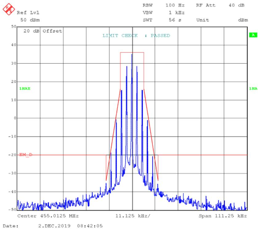
**FM,12.5kHz,Low Power – Frequency 455.0125 MHz:****99% Occupied & 26 dB Bandwidth**
