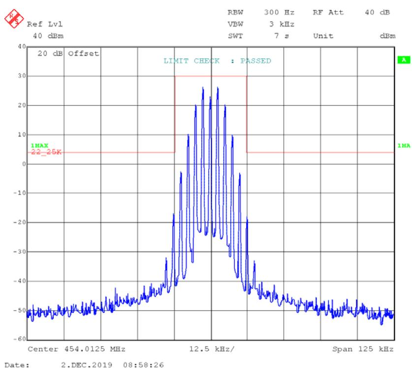
**4FSK,12.5kHz,High Power - Frequency 454.0125 MHz:****99% Occupied & 26 dB Bandwidth**
