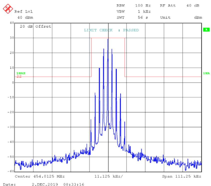
**FM,25kHz,High Power - Frequency 454.0125 MHz:****99% Occupied & 26 dB Bandwidth**
