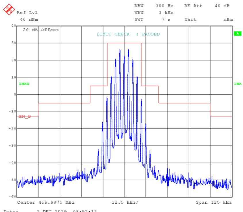
**part 74:****FM,12.5kHz,High Power - Frequency 455.0125 MHz:****99% Occupied & 26 dB Bandwidth**
