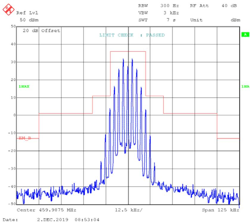
**FM,25kHz,Low Power - Frequency 459.9875 MHz:****99% Occupied & 26 dB Bandwidth**
