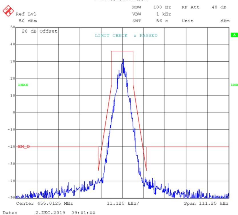
**4FSK ,12.5kHz, Low Power - Frequency455.0125 MHz:****99% Occupied & 26 dB Bandwidth**
