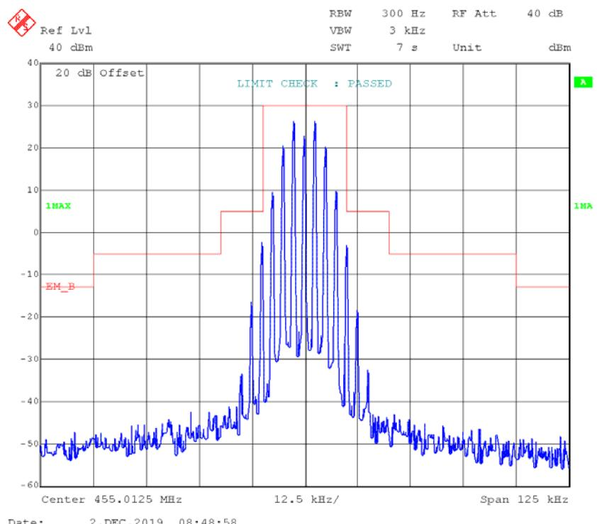
**4FSK ,12.5kHz, High Power - Frequency 455.0125 MHz:****99% Occupied & 26 dB Bandwidth**
