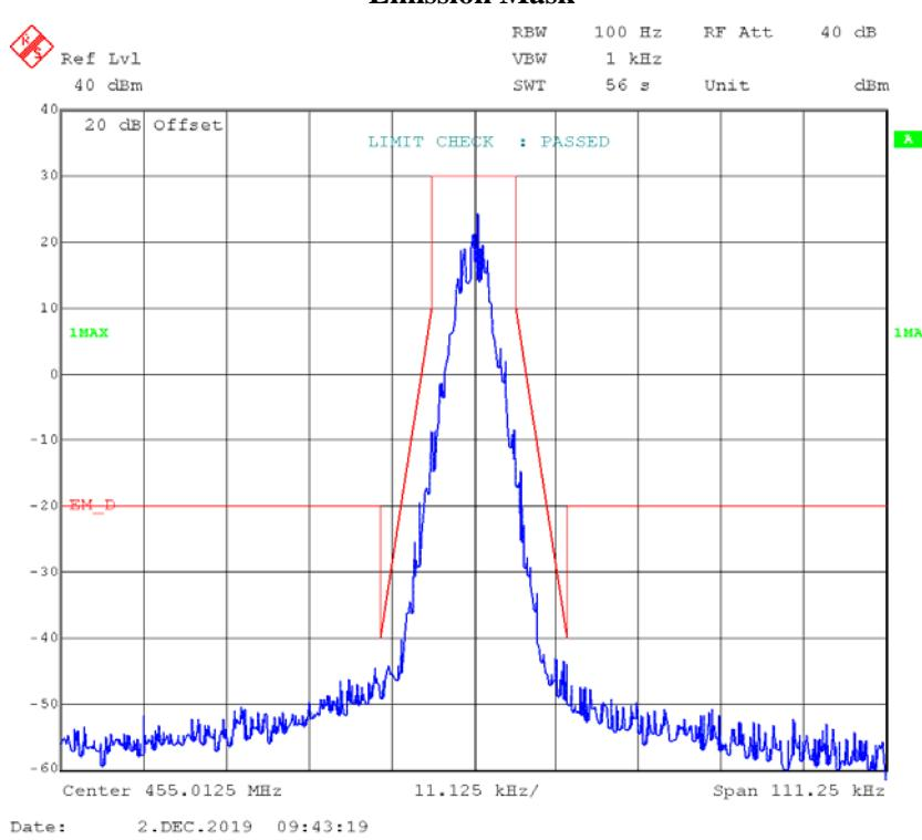
**part 22:****FM,12.5kHz,High Power - Frequency 454.0125 MHz:****99% Occupied & 26 dB Bandwidth**
