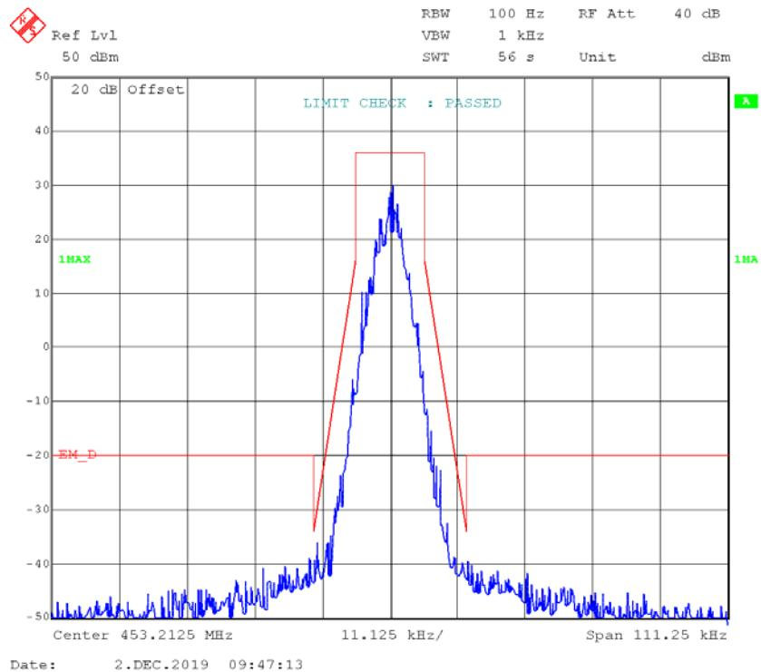
**4FSK,12.5kHz,Low Power - Frequency 453.2125 MHz:****99% Occupied & 26 dB Bandwidth**
