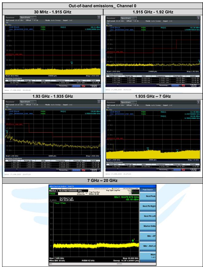
Note 1: The BS spurious out-of-band transmission level is below the indicated limit.
