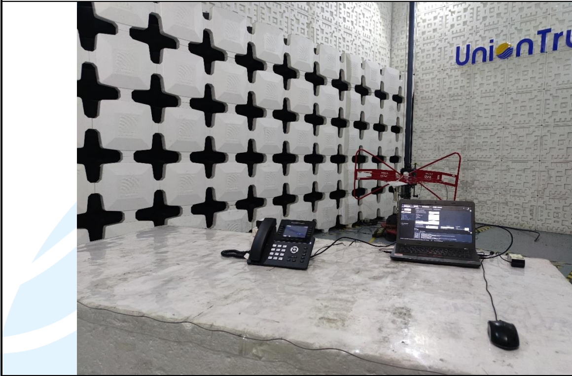
Radiated emission Test Setup (30 MHz~1 GHz)
