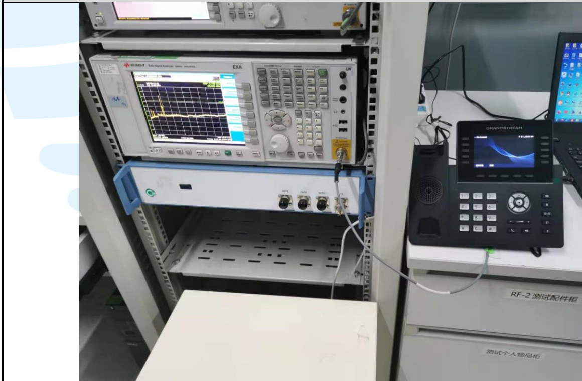
RF Conducted Test Setup
