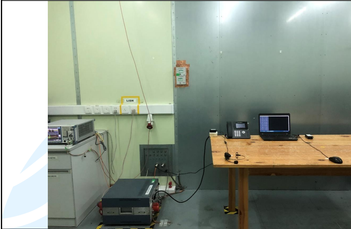
Conducted Emission Test Setup
