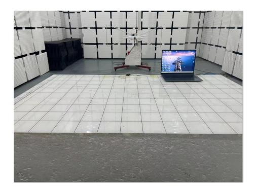
Set-up for Radiated Spurious Emission, Above 1GHz
