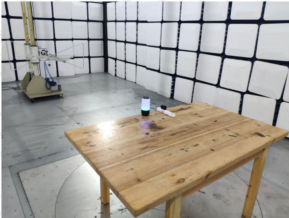
Photo of Radiation Emission Test
