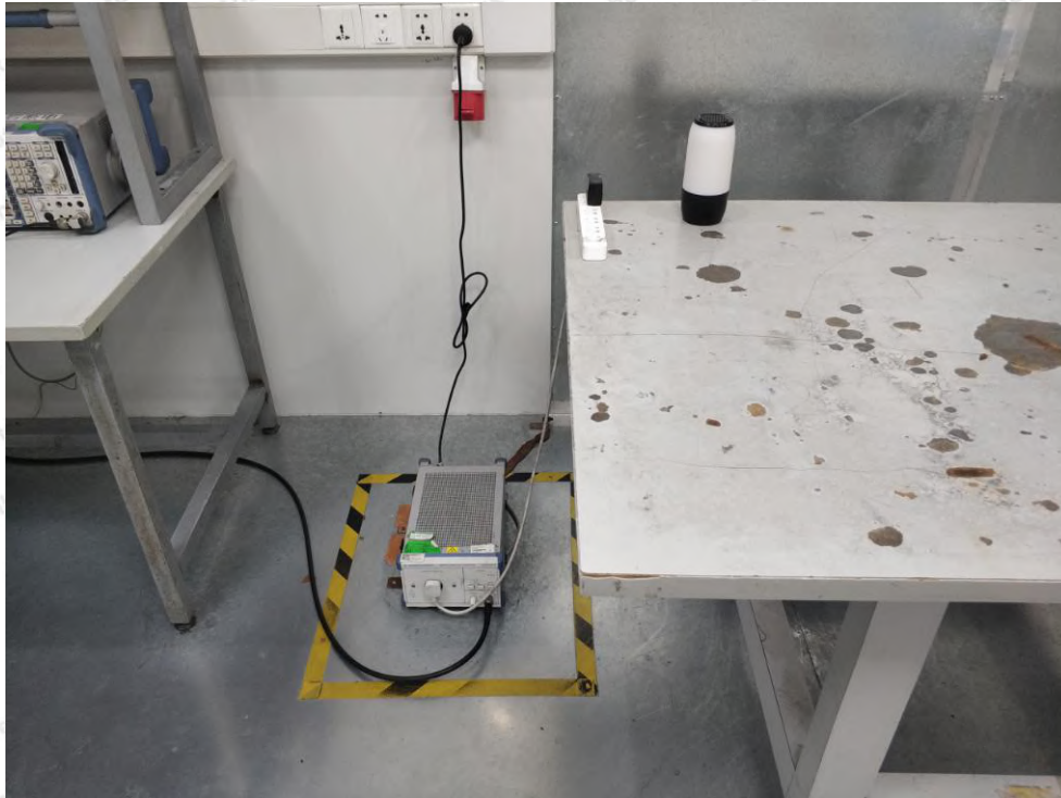
Photo of Conducted Emission Measurement
