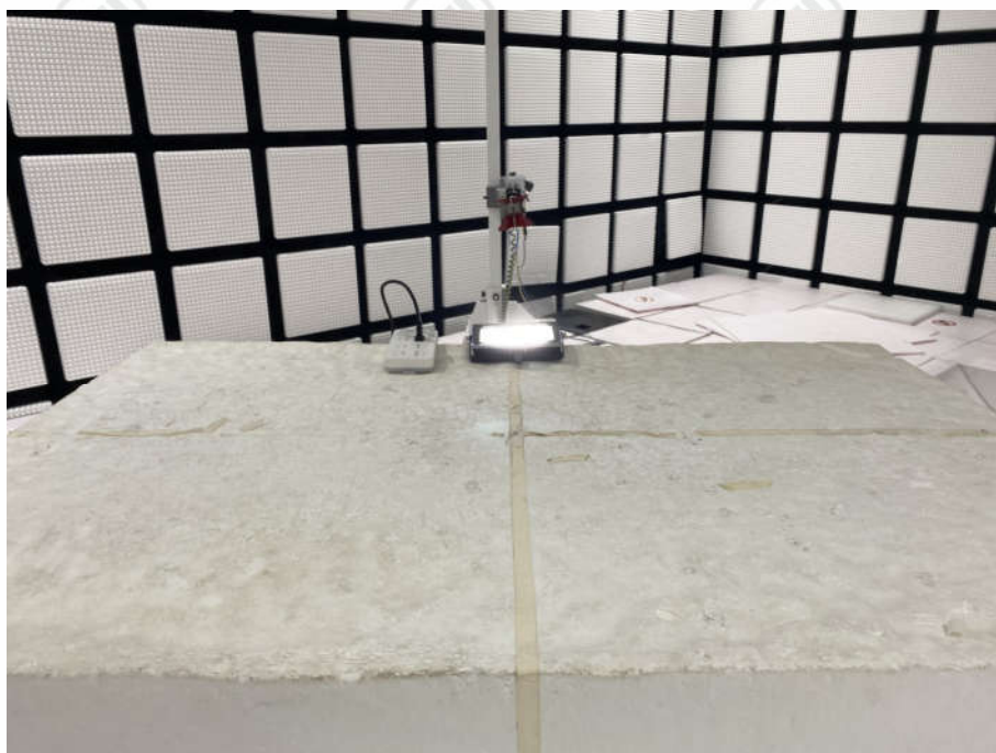
Radiated spurious emission Test Setup-2(Above 1GHz)
