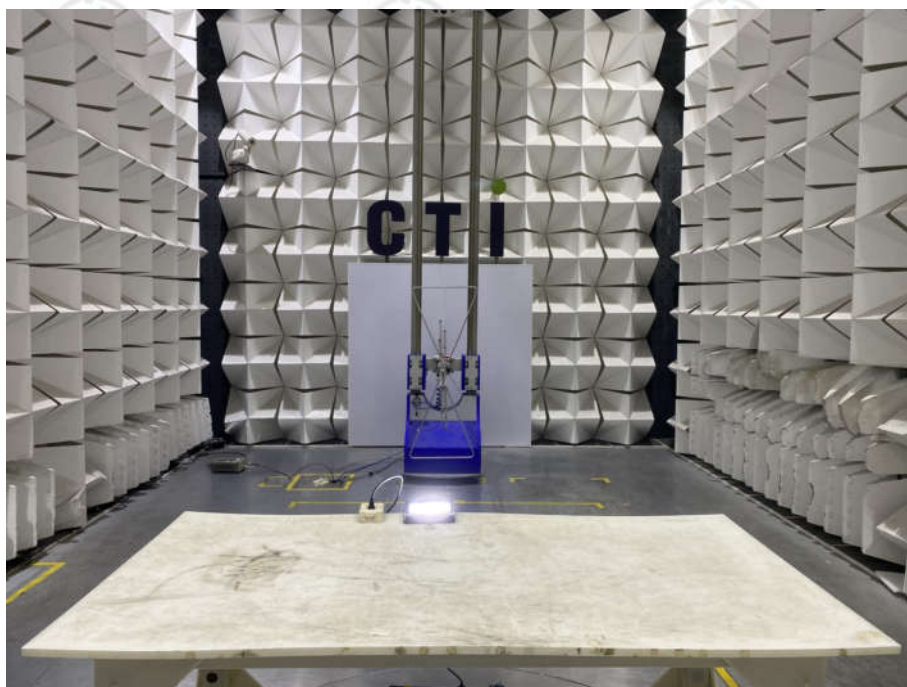
Radiated spurious emission Test Setup-1(Below 1GHz)
