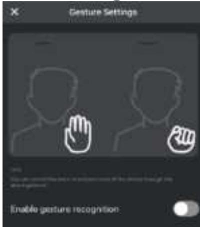
MAKI Live supports gesture recognition for hands-free zoom control. To use this feature, the camera must recognize your face and shoulders—either in a close-up or full-body framing.
