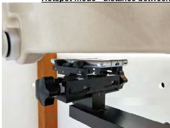
Fig.9 EUT Front side to flat phantom
