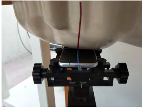
Fig.3 Right Head Section / Cheek-Touch Position
