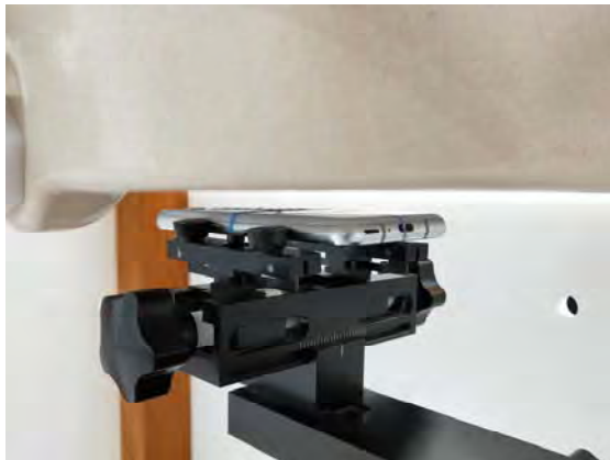
Fig.8 EUT Back side to flat phantom
