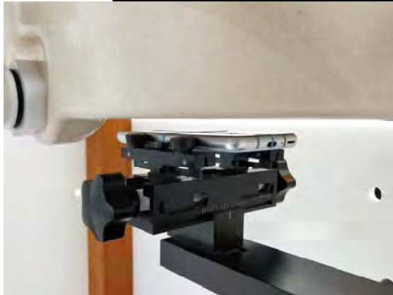
Fig.7 EUT Front side to flat phantom
