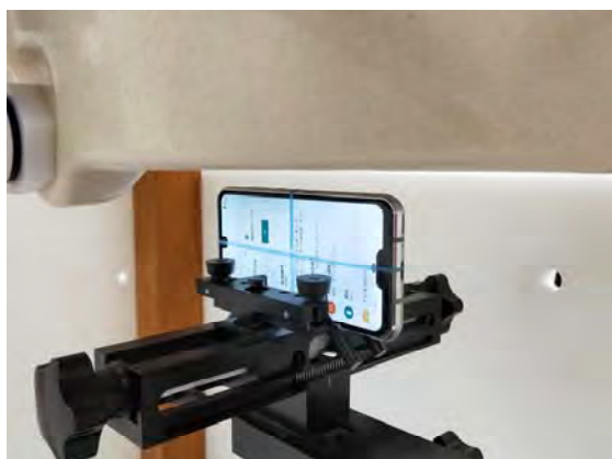
Fig.13 EUT Right side to flat phantom
