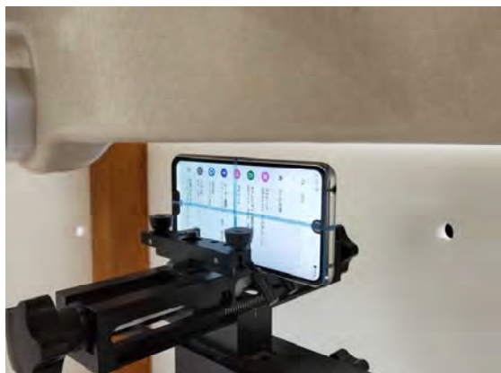
Fig.14 EUT Left side to flat phantom
